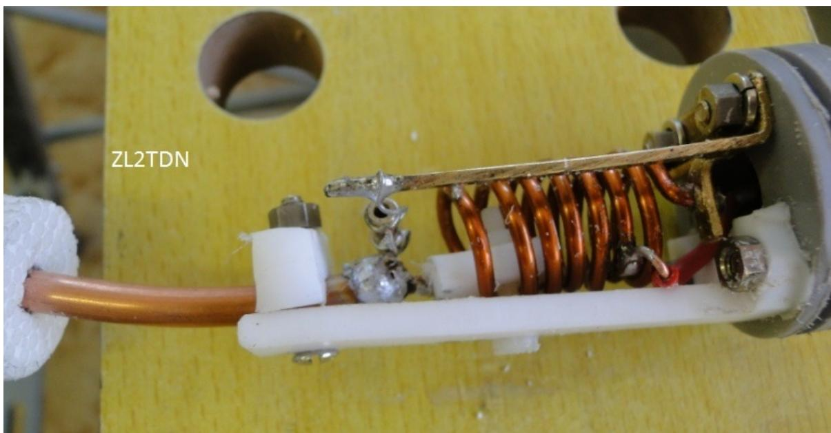
The coil is supported on a Teflon bracket and clamped to it by a nylon screw and a second piece of Teflon on the inside. The radiator tube is drilled through and bolted to the Teflon bracket.
