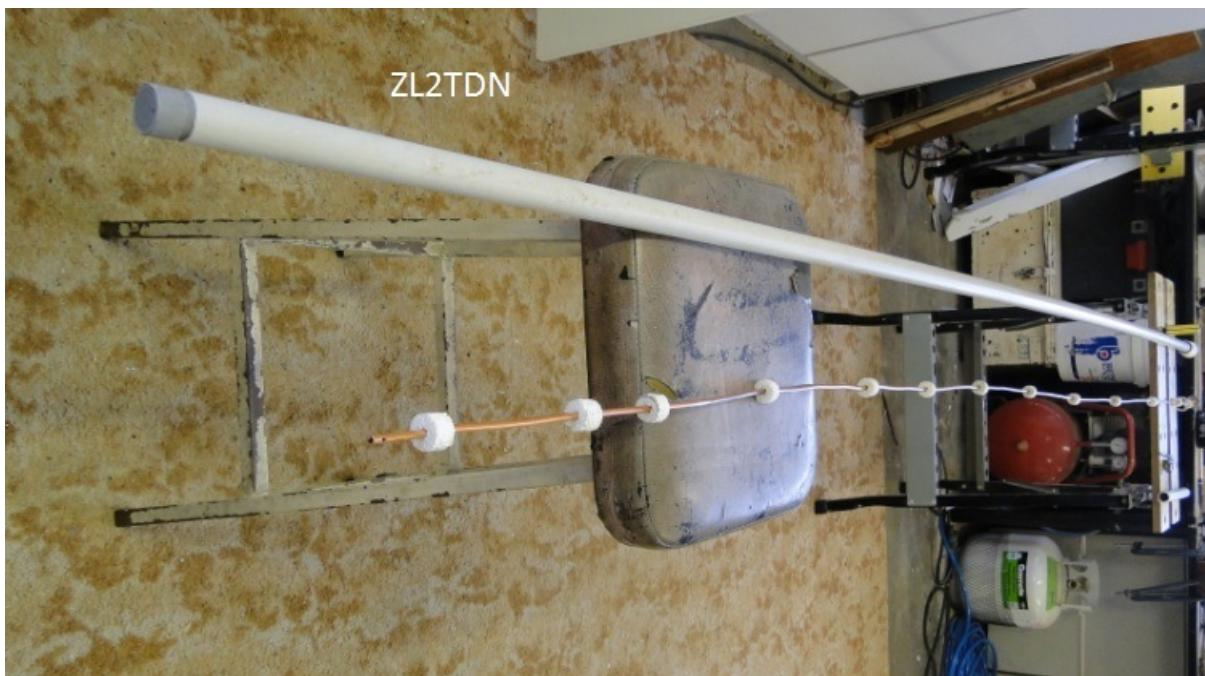
The antenna consists of a  $\frac{1}{2}$  wavelength of 3/16ths of an inch copper tubing (2804 mm) with polystyrene spacers every 200-250mm. This conductor is end fed by a parallel tuned circuit tuned to mid repeater band 53.450MHz. The incoming coax at 50 ohms is tapped on to the coil at about 1.5 to 1.75 of a turn from the bottom. The coil consists of about 7.5 turns tuned by a 22pF capacitor (500V), turns are double spaced, on a 13mm inside diameter.
