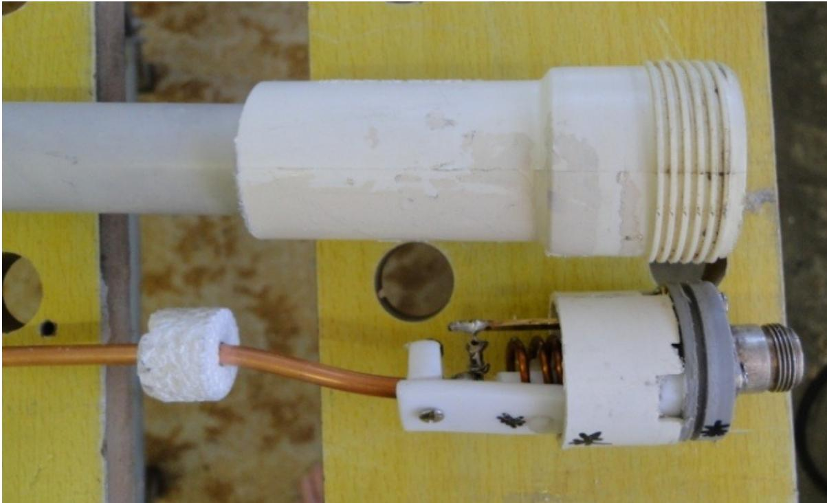
Here are the two outer parts, the packer sits in the bottom of the recess to clamp the gray socket support disk too with the clamp nut that's not shown here.
