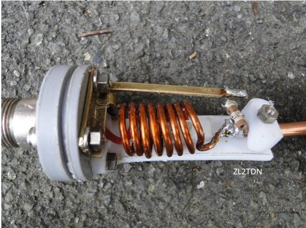
A 3mm hole between sets of bracket screws and the outside of the socket support disk holds a drain tube in case of condensation or leaks to enable water to escape.
