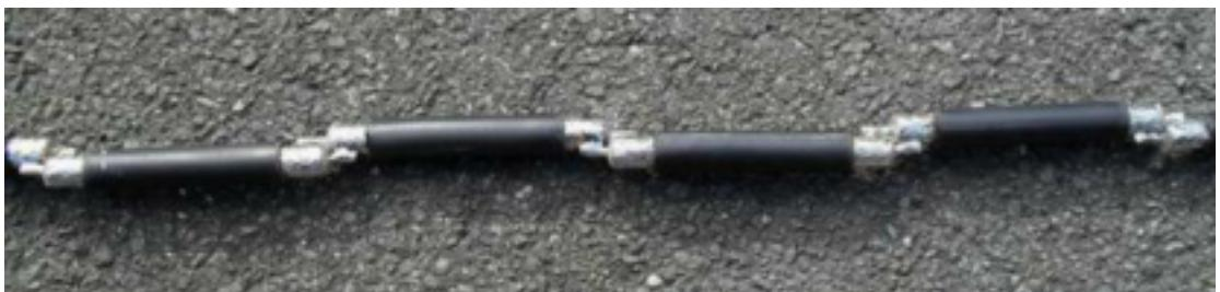
Silver plated wire was wrapped around the connection point for sweat soldering to the copper sleeve balun. A hot plumbers iron was used for a quick solder. This avoids over heating the coax braid and melting the coax dielectric. The antenna is now complete and ready for fitting to the PVC shroud.
