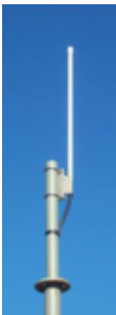
With a high speed cutting disk the resin knob was cut off. The tuning stub could now be adjusted. A silver plated 3mm diameter wire was used to fine tune the antenna. After tuning a new cap is resin filled and placed back on top. A small 2mm hole is required to release the air as it is pushed on. Tape around the hole until the resin has hardened.
