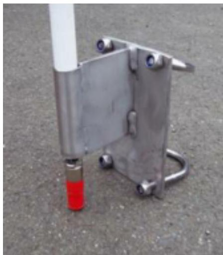
Phil ZL2HF designed a mounting sleeve socket fit for this purpose. This was the first antenna and was later replaced with a longer tail version for ease of connection to the LDF-450 Heliax feeder on site.
