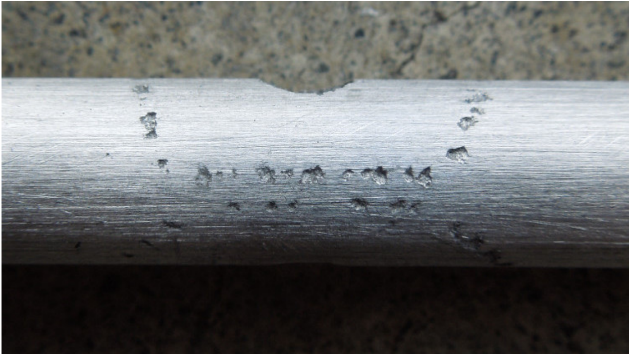
Picture-2: Dipole to boom corrosion pitting.
