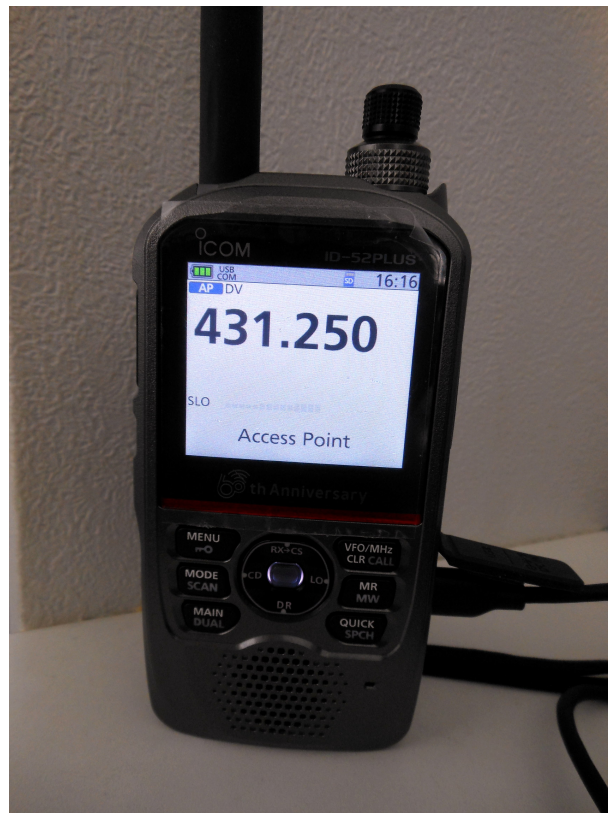
Picture-9 shows AP on UHF simplex USB connected to PC
